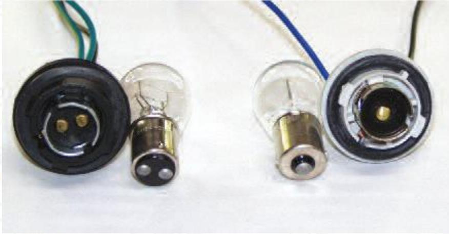
Two into one doesn't go - make sure the correct bulbs are fitted to the appropriate sockets
